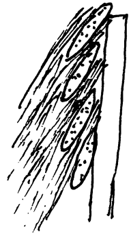
Method of Thatching (Note this should be sloping not vertical !!)
